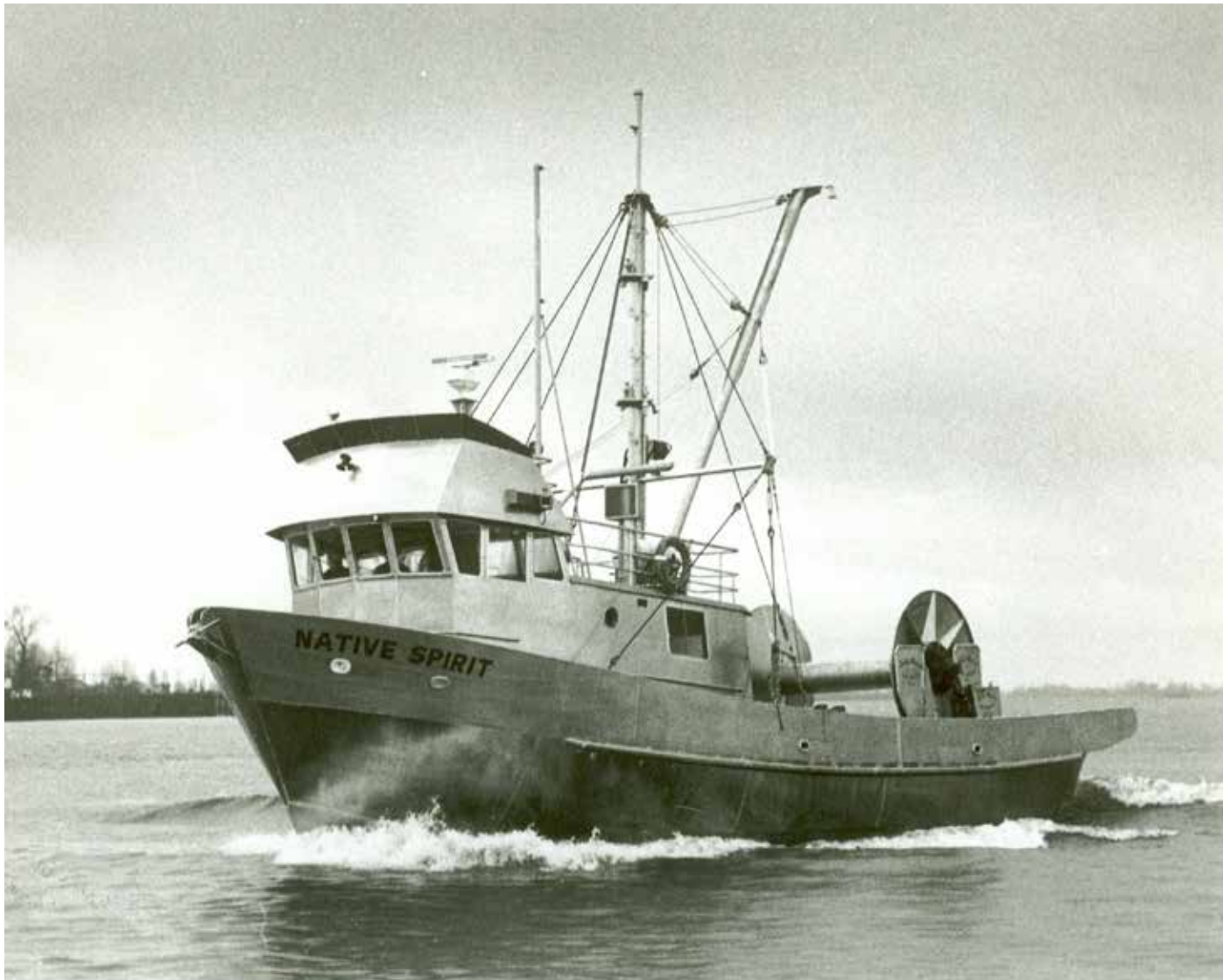
The brand new Native Spirit, Ron Sparrow Sr.'s first aluminium seine boat, on the Fraser River, c.1970-75. Collection of Ron and Vi Sparrow.
